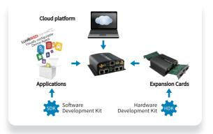
One of the major benefits of the product is flexible functionality which is achieved by supporting a wide range of plugin expansion cards: Wi-Fi client/AP, Micro-SD holder, Wi-Fi AP, LoRa WAN, industrial serial / serial / 2 - port serial, 1-port-Ethernet / 4-port-Ethernet / 4-port-PoE, BLE card, KNX, telematics, 4-ports USB, Developer Card with serial port for on-site connectivity and USB port for firmware update.
