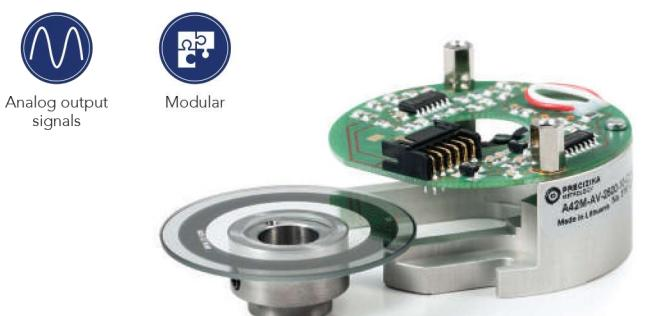
Photoelectric modular rotary encoder A42M is of incremental type and provides up to 25.000 output pulses per revolution. The absence of bearings and lubricants makes the encoder suitable for
