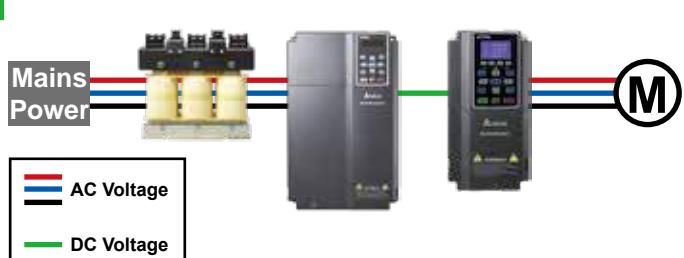
Provides the crane and hoist system excellent operation quality with reduced torque ripple, harmonic suppression, high power factors and energy saving performance with the power regeneration function.
