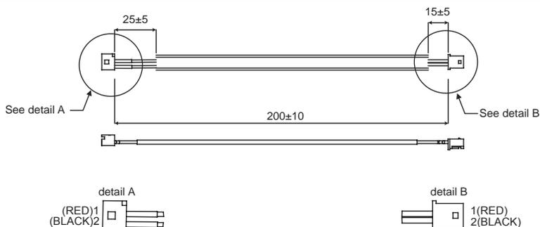
● **Battery Box Cord IW (Connects to CN8)** Units: mm
