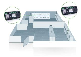
The practice of monitoring energy is becoming prevalent and modern data centers now include rack level monitoring at the design stage. The BFM-II monitors up to 54 single-phase loads and is ideal for PDU branch circuit monitoring, allowing for energy saving and offering high reliability.
